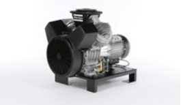
LF 10: Single-stage oil-free reciprocating compressor with a maximum working pressure of 10 bar (145 psi).
