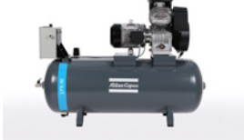
LT 10: Single-stage oil-lubricated reciprocating compressor with a maximum pressure of 10 bar (145 psi).
